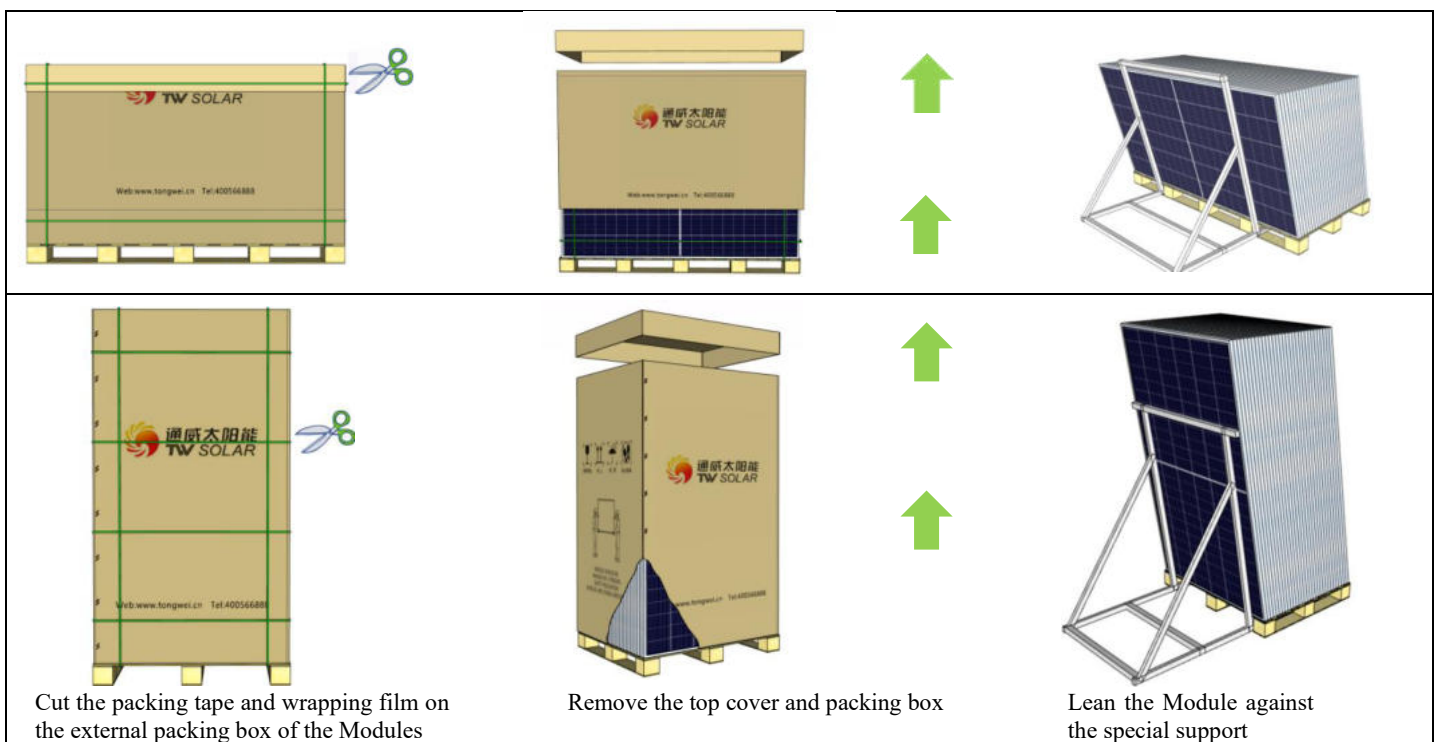
Figure 13 Schematic diagram of the unpacking procedure of the Module
