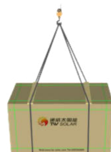
Figure 6 Schematic diagram of Module lifting
