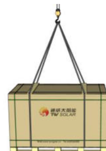
Figure 6 Schematic diagram of Module lifting
